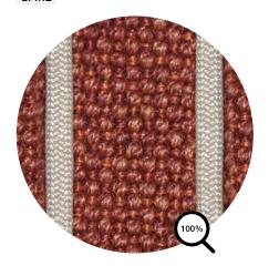
Fabric made entirely of polypropylene yarn, Ten Stars Yarn, exclusive patented, dyed in mass with an air flow texturization able to give the fabric a look and a softness comparable to natural fibers.
